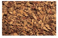
Wood chips produced by a company on Ibiza from fallen trees are a clean and cheap alternative to traditionally used diesel fuel. The equivalent energy to one liter of fuel is three kilograms of chips, which are cheaper and produce about 50% less harmful gasses when burned. However, this type of energy is not widely used on the island due to high installation costs. That being said, all public swimming pools on the island are heated with this type of fuel.
